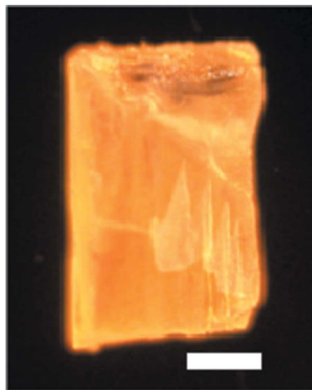
Figure 3 A photograph of a rectangular crystal of p -bromiodobenzene grown on a self-assembled monolayer. Scale bar = 0.5 mm.
